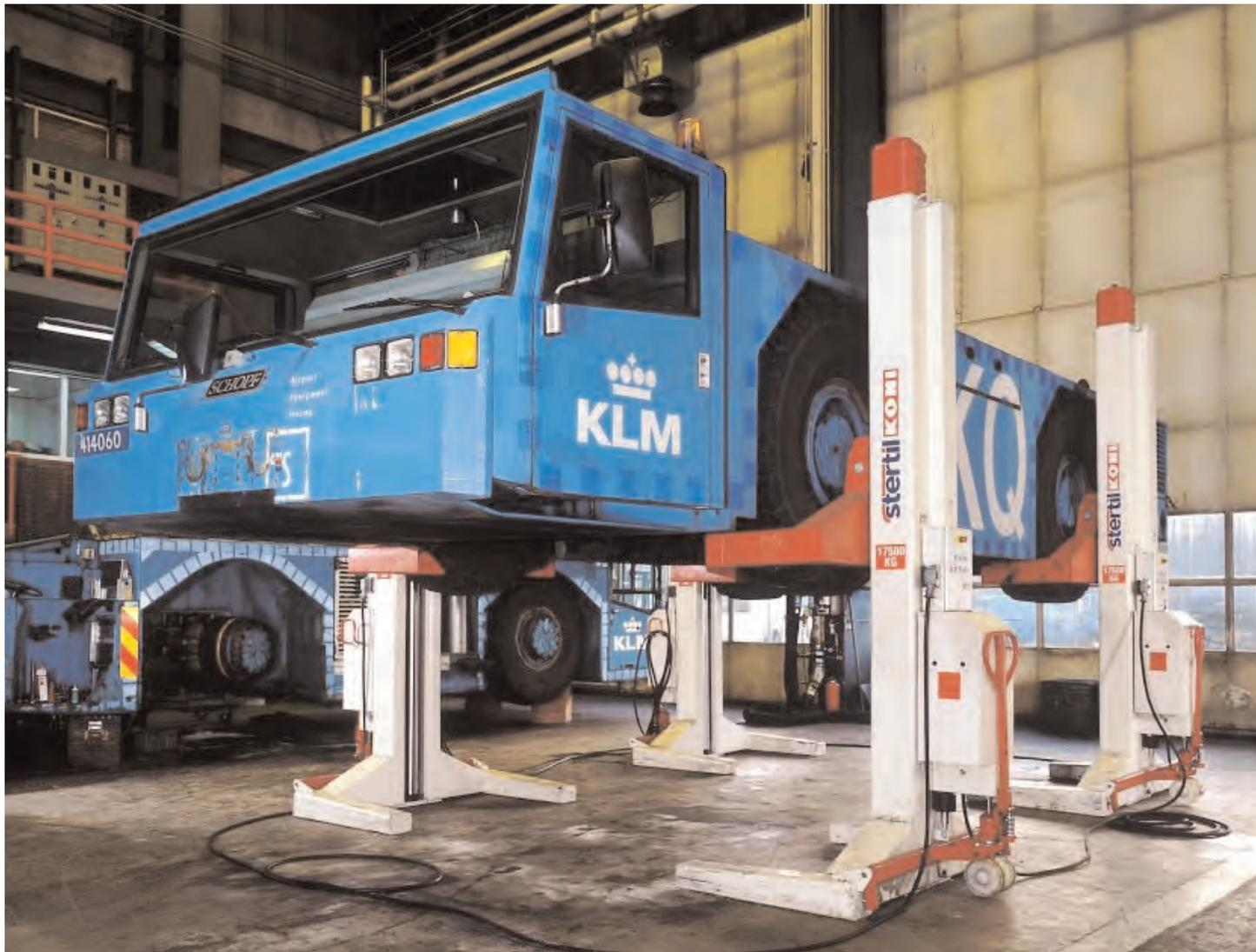
The flagship of our program is the mobile column lift, which is available with lifting capacity from 10,000 lbs. / 5.500 kg. up to 40,000 lbs. / 17.500 kg. per column. The advanced Stertil-Koni mobile column lift has earned its popularity because it has cleared the way for efficient and flexible workshop management.
