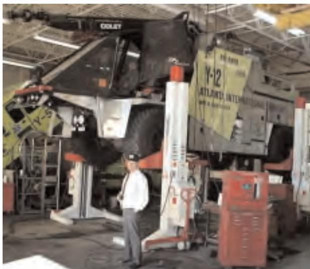
lifting columns in the world. The lifting height is over 2 metres, therefore it is comfortable to work with, even for tall people.
